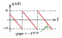
**Exercise 3**: A 100m transmission line has a velocity factor of 0.66. Plot the phase response of the cable over the frequency range 0 to 6 MHz.
