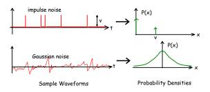
Signals that result from the sum of many small independent events have a probability distribution known as a Gaussian distribution. In communication systems this usually happens due to the sum of of voltages produced by the actions of very many individual photons, electrons or molecules.
