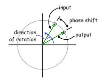
This phase shift is therefore a linear function of the delay with the delay defining the slope of the phase versus frequency curve.
