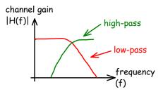
A band-pass channel is very common. A commonexample would be a transformer-coupled telephone line. Some band-pass channels result from attenuation by the channel but in other cases the band-pass nature of the channel intentional and is designed into the system to separate signals at different frequencies.
