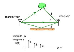
Since the each path length can be different, the delays for each path can be different. The different paths can add up constructively or destructively depending on the frequency and the delay. The frequency response can thus have peaks and nulls.
