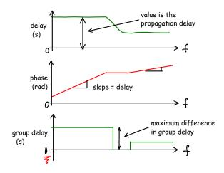
**Exercise 4**: A telephone line is being used to transmit symbols at a rate of 300 symbols/second. If the group delay must be less than 10% of the symbol period, what is the maximum allowable group delay?
