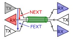
Note that the coupling between pairs in a cable happens throughout the length of the cable. The difference between NEXT and FEXT is in which receiver is affected (the near one or the far one), not where the coupling takes place.
