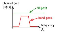
An all-pass channel has a flat amplitude response which would appear to have no effect on the signal. However filters with all-pass characteristics are sometimes used because of their effect on the channel's phase response.
