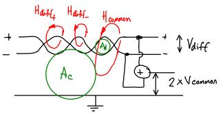
The area between the wires (Ad) is typically much smaller than the area between the wires and ground (Ac). In addition, the voltages induced on the twisted pair by the magnetic field (the parts of the field  $H_{diff+}$  and  $H_{diff-}$ ) will cancel out due to the twisting. Thus the noise induced on the differential voltage will be much less than the noise induced on the common-mode voltage. The receiver can ignore the common-mode voltage by subtracting the voltages on the two wires.
