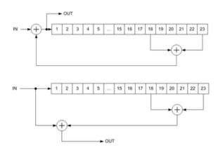
One problem with self-synchronizing scramblers is that an error in the received data pattern can result in multiple errors in the de-scrambled errors. This is called error propagation.
