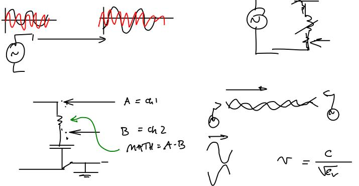
**Exercise 5**: An 800 MHz signal is output from a CATV amplifier at a power level of 10dBm. What power level would you expect at the other end of a 75m run of co-ax whose loss is specified as 24dB/100m at 800 MHz?
