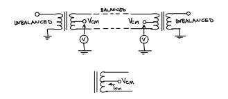
**Exercise 2:** If the common-mode circuit is used to carry 500mA, how much current flows through each half of the transformer secondary? What is the net effect on the flux in the transformer core?
