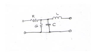
and the complete transmission line as an infinite sequence of the above blocks:
