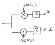
The receiver has to recover the phase of the carrier to accurately set the I and Q phases. This can be done, for example, by transmitting a preamble that has a known phase.
