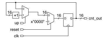
Use std\_logic for single-bit signals (those where the bus width is not shown) and unsigned for multi-bit signals. The block labelled +1 adds one to its input. Signals labelled with names in the schematic are entity inputs or outputs. You may choose any name(s) for signals within the architecture.
