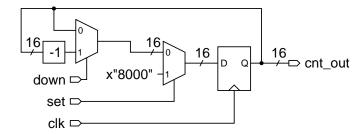
Use std\_logic for single-bit signals (those where the bus width is not shown) and unsigned for multi-bit signals. The block labelled -1 subtracts one from its input. Signals labelled with names in the schematic are entity inputs or outputs. You may choose any name(s) for signals within the architecture.
