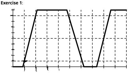
The diagram above shows an oscilloscope screen capture that includes one period of an *active-low* digital waveform. The scale on the horizontal axis is 20 ns per division. What are: the rise time, period, positive pulse width and duty cycle?
