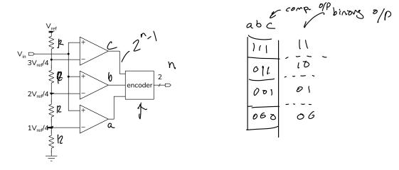
Draw a diagram showing the voltage ranges, the comparator outputs and the binary output for the 4-bit flash ADC above.
