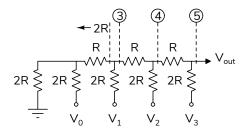
Show this. Assume  $V_1$  is set to  $V_{\rm ref}$  and all other inputs are zero (grounded). Find the output Thevenim resistance (resistance to ground at  $V_{\rm out}$  with  $V_1$  shorted) and voltage ( $V_{\rm out}$  with  $V_1 = V_{\rm ref}$ ). Hint: Do this at the labelled nodes.
