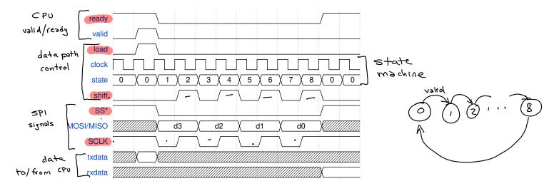
The diagram above shows the signals and state variable for a 4-bit SPI interface. The controller sequence generator states use a binary encoding. Write a state transition table for this state machine. Write Verilog expressions for the controller outputs.
