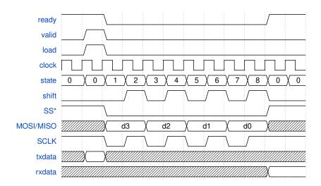
The diagram above shows the signals and state variable for a 4-bit SPI interface. The controller sequence generator states use a binary encoding. Write a state transition table for this state machine. Write Verilog expressions for the controller outputs.
