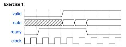
Mark the clock edges where data is transferred.
