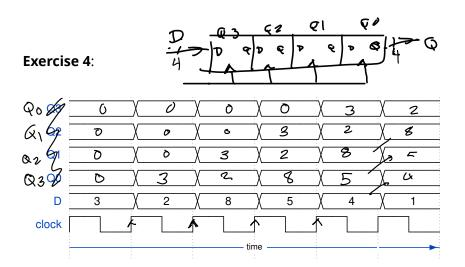
Fill in the diagram above for a 4-bit (N = 4) right-shift shift register. Assume the initial value is zero. Which bit is the oldest (first) value in the waveform? Which bit of the shift register holds the oldest value? **Exercise 5**: Draw a block diagram and write the Verilog for a circuit that sets an output named **detect** high when the sequence of values 1, 1, 0, 1 has appeared on an input named **in** on successive rising edges of the clock.
