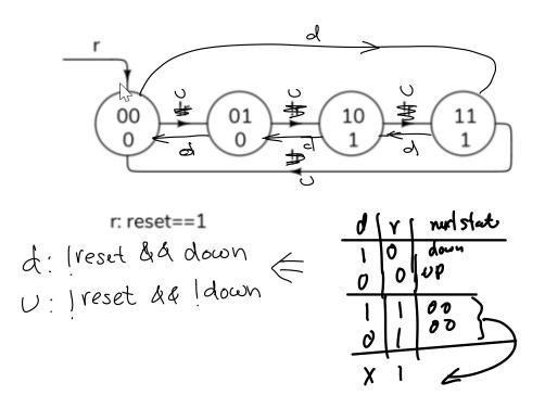
**Exercise 13**: How many bits need to be considered to detect a specific state when a binary encoding is used? How many need to be considered if a one-hot encoding is used?
