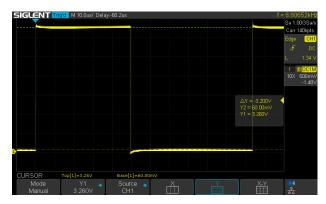
Record a screen capture of the 'scope display for your report. The display should show the voltage scale. Make sure the levels displayed make sense before taking a screen capture. Plug your USB flash drive into the USB socket on the front of the 'scope and press the "Print" button (below "Save") to capture the screen to your USB Flash drive<sup>4</sup>.
