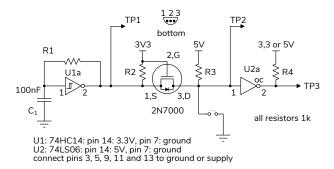
The Schmitt trigger inverter U1a is configured as an oscillator. When the output of the inverter is high, the capacitor charges up through a 1k resistor until it crosses the upper switching threshold  $(V_{T+})$ . Then the output switches off and discharges the capacitor through the resistor until the input crosses the lower switching threshold  $(V_{T-})$ .
