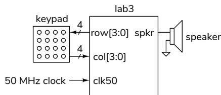
Your counters will use the 50 MHz clock on the CPLD board. The period of this clock is  $T = 1/50 \times 10^6 = 20$  ns.
