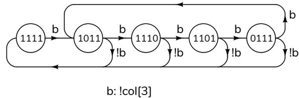
where the values in the circles show the values of the register **en**. The arrows labelled **b** show how **en** changes when  is pressed and the arrows labelled **!b** show how **en** changes when  is not pressed.
