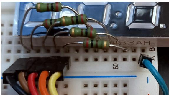
The active-low<sup>3</sup> digit-enable outputs are named `en[3]` through `en[0]` from left to right and the active-high segment-enable outputs are `a` through `g` (see the diagram above). Set `en[0]` low and the others high so that only the rightmost digit is enabled.
