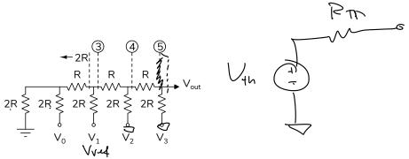
Assume  $V_1$  is set to  $V_{\rm ref}$  and all other inputs are zero (grounded). Find the Thevenim resistance (resistance to ground at  $V_{\rm out}$  with all  $V_i$  shorted) and voltage ( $V_{\rm out}$  with  $V_1=V_{\rm ref}$ ). Hint: Do this at the labelled nodes.
