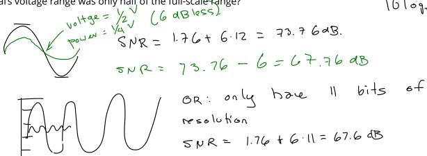
**Exercise 6**: A DAC outputs a digitized 1 kHz sine-wave signal. The analog output is analyzed and the power at 1 kHz is found to be 1 W while the power at all other frequencies adds up to 10 mW. What is the ENOB?
