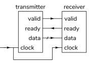
The transmitting device asserts a **valid** output when its data output is valid. The receiving device asserts a **ready** output when it is ready to accept data on the next clock  $edge^{1}$ . Data is transferred only on clock edges where both **valid** and **ready** are asserted.
