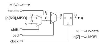
The shift register loads the eight **MOSI** bits to be transmitted from **txdata** when **load** is asserted. When **shift** is asserted a **MISO** bit shifts in on the
