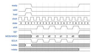
**Exercise 3:** Based on the diagram above, write a state transition table for an SPI interface controller that transfers four bits at a time. Include an idle state. In which states are SCLK and  $\overline{SS}$  asserted?
