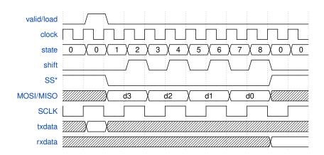
Based on the diagram above, write a state transition table for an SPI interface controller that transfers four bits at a time. Include an idle state. In which states are **SCLK** and **SS** asserted?
