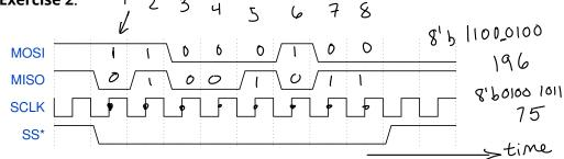
The diagram above shows a transfer over an SPI bus. How many bits of data are transferred? What is the value, in decimal, of the data transferred from the master to the slave? From the slave to the master?
