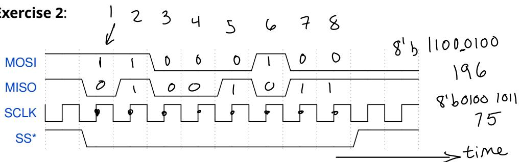
The diagram above shows a transfer over an SPI bus. How many bits of data are transferred? What is the value, in decimal, of the data transferred from the master to the slave? From the slave to the master?
