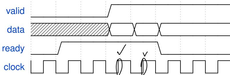
Mark the clock edges where data is transferred.
