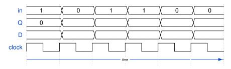
Fill in the diagram above for a 4-bit (N = 4) right-shift shift register. Assume the initial value is zero. Which bit is the oldest (first) value in the waveform? Which bit of the shift register holds the oldest value? **Exercise 3**: Draw a block diagram and write the Verilog for a circuit that sets an output named **detect** high when the sequence of values 1, 1, 0, 1 has appeared on an input named **in** on successive rising edges of the clock.
