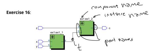
Identify the following in the diagram above: component names, component "instance names," component port names, module port names. Label the signal **t** in the schematic.
