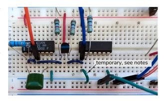
Use the 5 V and 3.3 V supplies from the CPLD board (the ground, 3.3 V and 5 V pins are on the pin headers at the upper right of the board):
