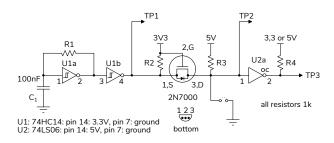
The Schmitt trigger inverter U1a is configured as an oscillator. When the output of the inverter is high, the capacitor charges up through a 1k resistor until it crosses the upper switching threshold  $(V_{T+})$ . Then the output switches off and discharges the capacitor through the resistor until the input crosses the lower switching threshold  $(V_{T-})$ .
