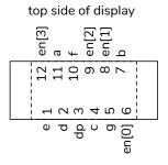
Review the schematic above and notice how the LEDs are connected. This is a common-cathode display so you must set the pin for a segment (A-G) high and the desired digit enable (DIG1 through DIG4) low to turn on that LED segment. Note that only one digit can be displayed at a time.
