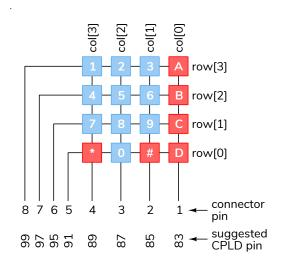
The photo below shows how the keypad is connected:
