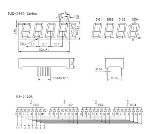
The display pinout is:
