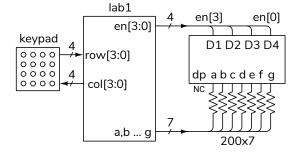
Your circuit should display one of the last three digits of your BCIT ID in the rightmost digit position when the keypad buttons 1, 4, and 7 are pressed. For
