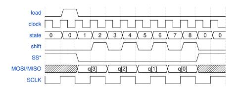
Based on the diagram above, write a state transition table for an SPI interface controller that transfers four bits at a time. Include an idle state. In which states are **SCLK** and **SS** asserted?
