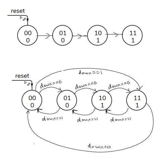
**Exercise 2**: Show the state transition diagram and table for a 2-bit counter with reset, enable, and down inputs. Reset should have priority. Write the Verilog.
