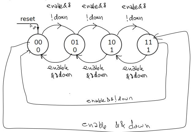
$$\begin{array}{c|c} count & reset enable down & count \\ \hline \chi \chi & 1 & \chi & 0 & 0 \\ \hline n & 0 & 0 & \chi & h \\ \hline 1 & 0 & 1 & 0 & 0 \\ \hline 1 & 0 & 1 & 0 & 0 \\ \hline 0 & 0 & 1 & 1 & 11 \\ \hline n & 0 & 1 & 0 & -1 \\ \hline n & 0 & 1 & 1 & h-1 \end{array}$$
