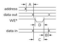
Write the appropriate letter from the timing diagram on the left for each of the following RAM timing specifications:
