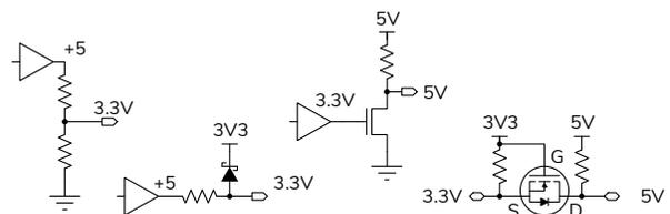
If the high output voltage is too high, a resistive voltage divider or a current-limiting resistor and a (Schottky) diode clamp<sup>3</sup> to the lower supply voltage can be used. If the high output voltage is too low<sup>4</sup>, an open-collector output or n-channel MOSFET and pull-up resistor can be used.
