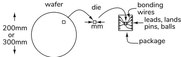
There are a wide variety of packages available. You've used dual-in-line (DIP) packages which are suitable for "through-hole" mounting. The IC on your CPLD or FPGA board uses a TQFP (thin quad flat package) which is suitable for "surface-mount" circuit boards. Higher densities can be achieved with BGA (ball-grid array) packages which have a rectangular array of connecting solder balls on the bottom.
