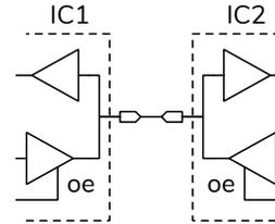
To connect multiple outputs in parallel we must ensure that only one output is enabled at a time. Otherwise two devices could try to drive the same net to different levels. This is called contention and results in excessive current and, potentially, damage.
