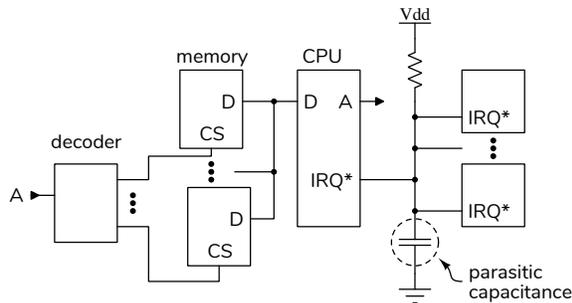
**Exercise 5:** What are the active-state current and the RC time constant for a wired-or interrupt-request line using a 10kΩ resistor pulling up a circuit with 50 pF capacitance to 3.3 V?
