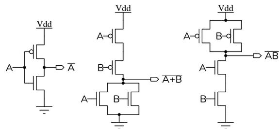
In each case the appropriate combination of NMOS transistors are turned on to pull the output low. Otherwise the PMOS transistor(s) pull the output high.
