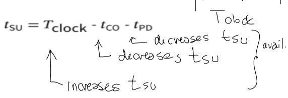
**Exercise 3**: For a particular circuit  $f_{\text{Clock}}$  is 50 MHz,  $\hat{\text{LCO}}$ . is 2 ns (maximum), the worst-case (maximum) PD. in a circuit is 15 ns and the minimum setup time requirement is 5 ns. What is the setup time slack? Will this circuit operate reliably? If not, what it the maximum clock frequency at which it will?
