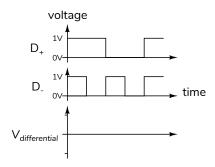
**Exercise 4:** The diagram above shows the voltages on a differential pair. The differential voltage is  $V_{\rm differential}=D_+-D_-$ . Draw the differential voltage waveform.
