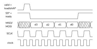
**Exercise 2:** Based on the diagram above, write a state transition table for an SPI interface controller that transfers four bits at a time. Include an idle state. In which states are SCLK and  $\overline{SS}$  asserted?
