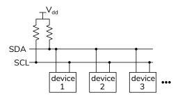
Often, one device is a master and "polls" the slave. After each poll the master turns off its driver and the slave turns on its driver for the duration of the response. However, there are also interfaces (including I<sup>2</sup>C) where multiple devices can contend to become the bus master using an "arbitration" protocol.
