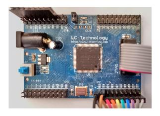
The four 20-pin headers will be used to connect components such as an LED display and a keypad. The CPLD pin numbers connected to each header pin are marked on the PCB.
