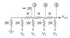
Show this. Assume  $V_1$  is set to  $V_{\text{ref}}$  and all other inputs are zero (grounded). Find the Thevenim resistance (resistance to ground at  $V_{\text{out}}$  with all  $V_i$  shorted) and voltage ( $V_{\text{out}}$  with  $V_1 = V_{\text{ref}}$ ). *Hint: Do this at the labelled nodes.*
