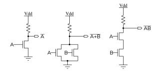
When one (for NOT), either A or B (for OR) or both A and B for (AND) inputs are high ( $>V_{\rm th}$ ) the transistors pull the output low. The resistor (typically implemented with a transistor structure) pulls the output high otherwise.
