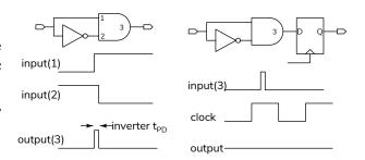
Glitches on IC outputs increase power consumption and noise. Increased power consumption results from charging and discharging interconnect capacitances for each glitch. The short glitch duration allows it to be readily coupled to other signals and to be radiated. This increases noise.
