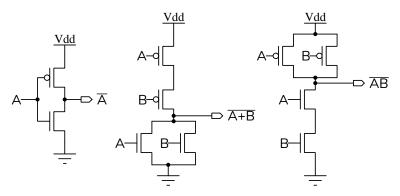
In which direction does the output current flow when the output is high? When it is low? Which transistors in the NAND circuit are on (conducting) in each case?
