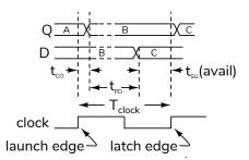
Q becomes valid  $t_{CO}$  after the first ("launching") rising clock edge. After  $t_{PD}$ , the propagation delay through the combinational logic, D will have a correct and valid logic level.
