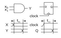
These main contribution to these delays is the time required to charge the parasitic capacitances of transistors and the connections between them. **Exercise 3:** Is  $t_{PD}$  a requirement or a guaranteed response?
