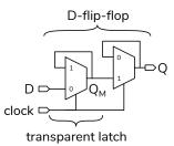
When the clock input is low, the output of the first multiplexer follows the input – the latch is "transparent". When the clock input is high, the output level is fed back to the input and held at that level. The second multiplexer is transparent when the clock is high and holds the value captured by the first multiplexer when the clock is low. This results in the output only changing on the rising edge of the clock.
