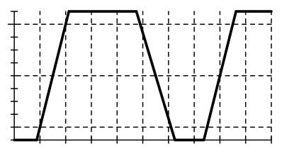
The diagram above shows an oscilloscope screen capture that includes one period of an *active-low* digital waveform. The scale on the horizontal axis is 20 ns per division. What are: the rise time, period, positive pulse width and duty cycle?
