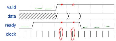
Mark the clock edges where data is transferred.
