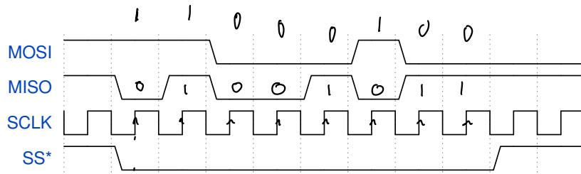
The diagram above shows a transfer over an SPI bus. How many bits of data are transferred? What is the value, in decimal, of the data transferred from the master to the slave? From the slave to the master?
