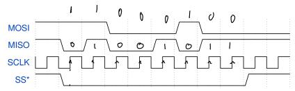
The diagram above shows a transfer over an SPI bus. How many bits of data are transferred? What is the value, in decimal, of the data transferred from the <u>master to the slave</u>? From the slave to
