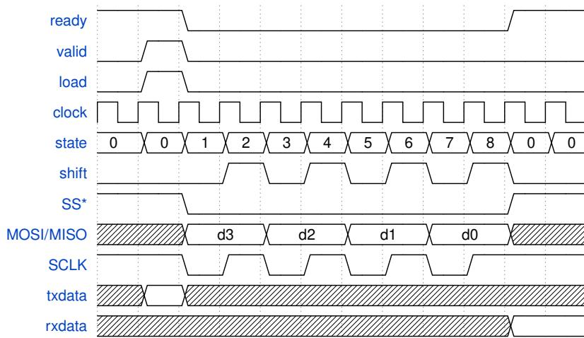
Based on the diagram above, write a state transition table for an SPI interface controller that transfers four bits at a time. Include an idle state. In which states are **SCLK** and **SS** asserted?
