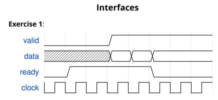
Mark the clock edges where data is transferred.
