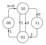
**Exercise 7:** For which states would a **fell** output be asserted? A **rose** output? Draw the schematic and write the Verilog for this state machine. Assume an input **in** and a 2-bit register **bits** that holds the two most recent input values.
