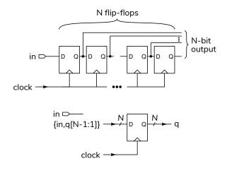
**Exercise 1:** The example above is an N-bit shift register that shifts the bits right. Draw a block diagram and write the Verilog for a 6-bit shift register that shifts left.
