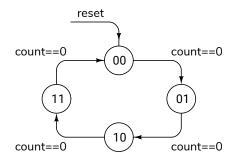
**Exercise 10:** Write the state transition table for this state machine. The state transition table for the timer is:
