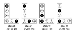
Delays are implemented by decrementing **count** on each edge of a 1 Hz clock. When **count** reaches zero the **state** register is loaded with the next state and the counter register is loaded with the duration of this next state.
