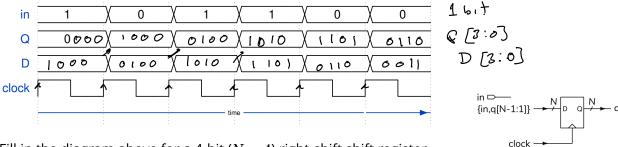
Fill in the diagram above for a 4-bit (N=4) right-shift shift register. Assume the initial value is zero. Which bit is the oldest (first) value in the waveform? Which bit of the shift register holds the oldest value?
