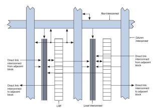
Complex software is required to fit a design into an FPGA and route the signals between logic elements. Because of the multiple levels of interconnect the propagation delays are harder to predict than for a CPLD. Even if there is sufficient logic, some designs may not 'fit' into an FPGA because of insufficient routing resources.
