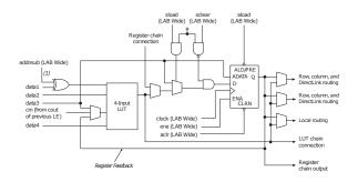
Each LE implements combinational logic using a 4 bit in, 1 bit out look-up table (LUT). The LUT output is fed to a single flip-flop. Programmable multiplexers allow groups of LE's to be efficiently configured into a wide range of more-complex logic functions such as registers and adders.
