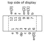
Review the schematic above and notice how the LEDs are connected. This is a multiplexed commoncathode display so you must set the pin for a segment (A-G) high *and* the desired digit enable (DIG1 through DIG4) low to turn on that LED segment on that digit. Only one digit can be displayed at a time because the segment enables are shared by all digits.
