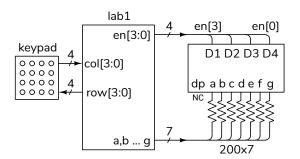
Your circuit should display one of the rightmost four digits of *your* BCIT ID in the rightmost digit position when keys 1 through A are pressed. For example, if your BCIT ID were A00123456 then when 1 is pressed the rightmost LED should display 3, when 2 is pressed the rightmost LED should display 4, etc. Otherwise, nothing should be displayed.
