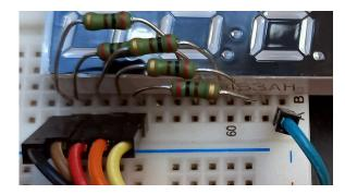
The active-low<sup>3</sup> digit-enable outputs are named en[3] through en[0] from left to right and the active-high segment-enable outputs are a through g (see the diagram above). Set en[0] low and the others high so that only the rightmost digit is enabled.
