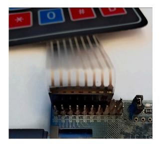
The columns are connected to inputs configured with internal pull-up resistors<sup>2</sup>. Your code must set the top row low and the others high.
