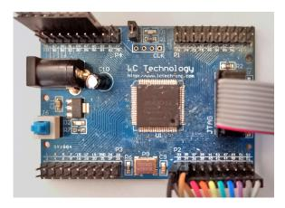
The CPLD has 100 pins. The board has four 20pin headers that allow you to connect to most of the CPLD pins. CPLD pin numbers are marked next to each header pin. You will use these pins to connect components such as an LED display and a keypad.
