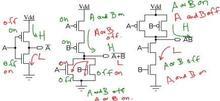
Which transistors are on when the output is high? When it is low? In which direction does the output current flow in each case?
