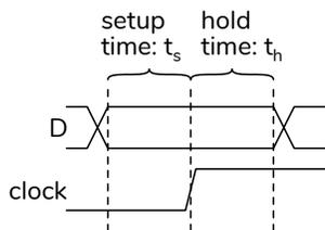
**setup time** the D input must be at a valid logic level for at least  $t_S$  before the rising edge of the clock
