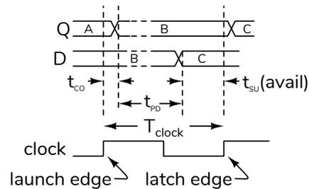
Q becomes valid  $t_{CO}$  after the first (“launching”) rising clock edge. After  $t_{PD}$ , the propagation delay through the combinational logic, D will have a correct and valid logic level.
