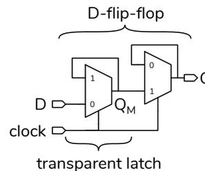
When the clock input is low, the output of the first multiplexer follows the input – the latch is “transparent”. When the clock input is high, the output level is fed back to the input and held at that level. The second multiplexer is transparent when the clock is high and holds the value captured by the first multiplexer when the clock is low. This results in the output only changing on the rising edge of the clock.
