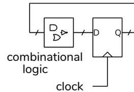
On the rising edge of the clock the flip-flop output changes, and it takes  $t_{PD}$  for the changes to fully propagate through all of the logic.
