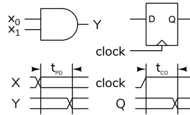
These main contribution to these delays is the time required to charge the parasitic capacitances of transistors and the connections between them.
