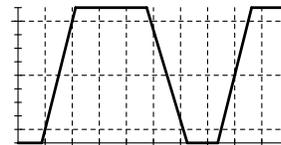
**Exercise 1:** The diagram above shows an oscilloscope screen capture that includes one period of an *active-low* digital waveform. The scale on the horizontal axis is 20 ns per division. What are: the rise time, period, positive pulse width and duty cycle?
