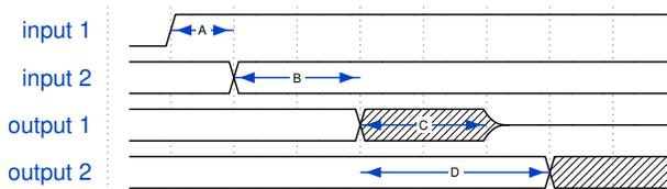
**Exercise 2:** Label the specifications A through D as requirements or guaranteed responses. Which specifications are measured to a signal being in a high-impedance state? Which are measured from a rising edge only? From either?
