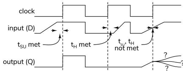
To avoid metastability we must ensure the voltage at the latch input is at valid level long enough to drive the latch output to a valid voltage level before the rising edge of the clock. The time required for this is called the “setup” time,  $t_{SU}$ .
