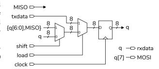
The shift register loads the eight MOSI bits to be transmitted from txdata when load is asserted. When shift is asserted a MISO bit shifts in on the right and a MOSI bit shifts out on the left. At the end of the transfer the eight received MISO bits can be read in parallel from the shift register on rxdata.
