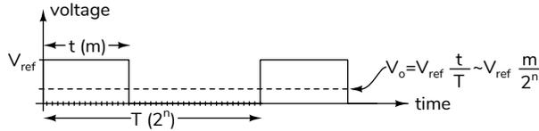
When this waveform is low-pass filtered so that only the DC (zero-frequency) component remains, the output is a voltage proportional to the high level voltage ( $V_{ref}$ ) and the duty cycle.
