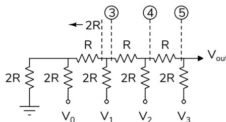
$$V_{out} = \left( \frac{V_3}{2} + \frac{V_2}{4} + \frac{V_1}{8} + \frac{V_0}{16} \right)$$
