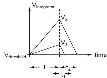
A dual-slope ADC integrates the input for a fixed duration ( $T$ ) and measures the time required to integrate a negative reference voltage until the integrator is discharged. The ratio  $t/T$  is the ratio of  $V_{in}/V_{ref}$ . This approach eliminates the dependence on several analog components (integrator  $R$  and  $C$ , comparator thresholds, and clock rates).
