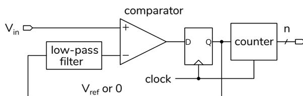
A Sigma-Delta ADC requires clock rates much higher than (e.g. 100 times)<sup>3</sup> the sampling rate but is inexpensive because it does not require accurate analog components (e.g. the accurate resistors in the R-2R network used in a SAR ADC).
