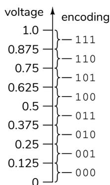
The “resolution” of an ADC can refer to either the number of bits,  $n$ , (e.g. “a 10-bit resolution ADC”) or the difference between adjacent voltage levels,  $\Delta$  (e.g. “a resolution of 1 mV”). Units determine which definition is being used.
