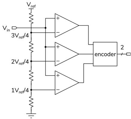
This is the fastest type of ADC – the sampling rate is equal to the clock rate – but it is the most expensive as the complexity increases exponentially with  $n$ .
