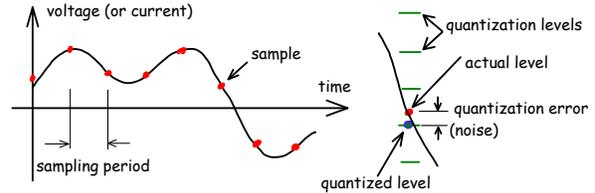
A digitized signal can be converted to a continuous signal by generating a step-like waveform with the required levels at the required sampling rate. The circuit that does this is called a digital-to-analog converter (abbreviated as DAC or D/A).
