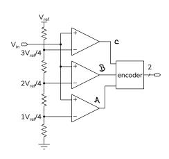
Draw a diagram showing the voltage ranges, the comparator outputs and the binary output for the 4-bit flash ADC above.
