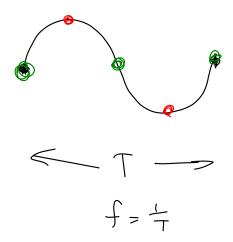
**Exercise 2**: What minimum sampling rate would be required to digitize a 10 kHz square wave if you wanted to include frequency components up to the 7'th harmonic (at 70 kHz)?
