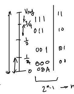
**Exercise 11**: A SAR ADC using a 4-bit DAC with a full-scale range of 0 to 7.5 V digitizes a 5.25 V signal. What voltages will the DAC output?
