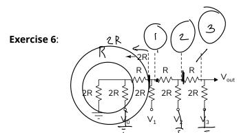
Assume  $V_1$  is set to  $V_{\text{ref}}$  and all other inputs are zero (grounded). Find the Thevenim resistance (resistance to ground at  $V_{\text{out}}$  with all V shorted) and voltage (V with V - V)
