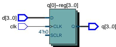
Note the use of “non-blocking assignment” (`<=`) in `always_ff` statements. As with the blocking assignment (`=`), the leftmost bits are dropped if the RHS is wider than the LHS.
