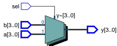
Conditional operators can be used to concisely describe trees of multiplexers. In the absence of parentheses a sequence of conditional operators is evaluated from left to right.
