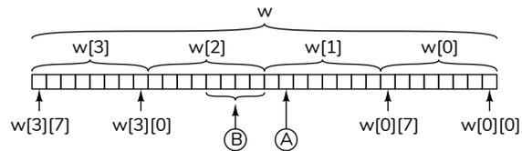
**Exercise 18:** How would you specify the bit marked A in the diagram above? The bits marked B? The least-significant byte?
